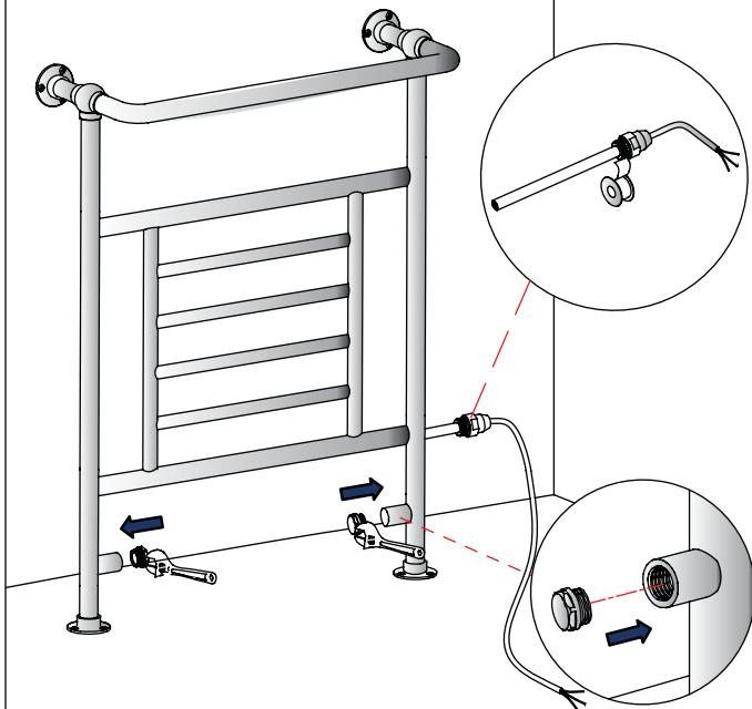
6 Connect to the electric supply via a fused spur. Then check for leaks. At all times follow the installation instructions supplied with the Summer Electric Heating kit. All electric work must be done by a suitably qualified person.
